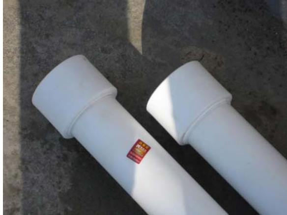
PP pipe material of the vacuum pipe-line
